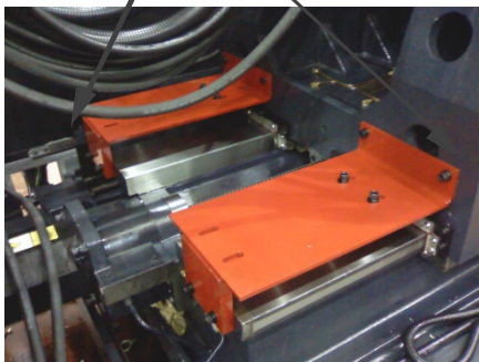
<Fixture between column and column bed>
