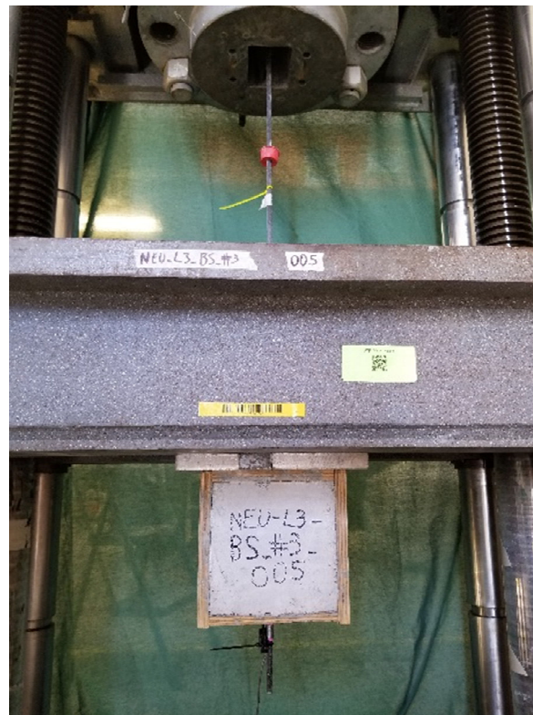
Figure 11.2 – Bond strength test set-up
